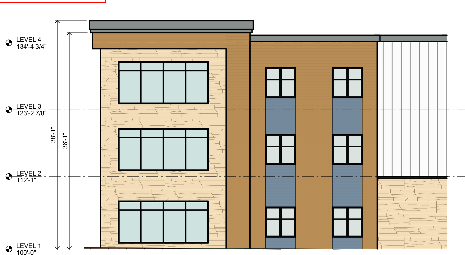
B2 CARE CENTER - ELEVATION 2 1/8" = 1'-0"
