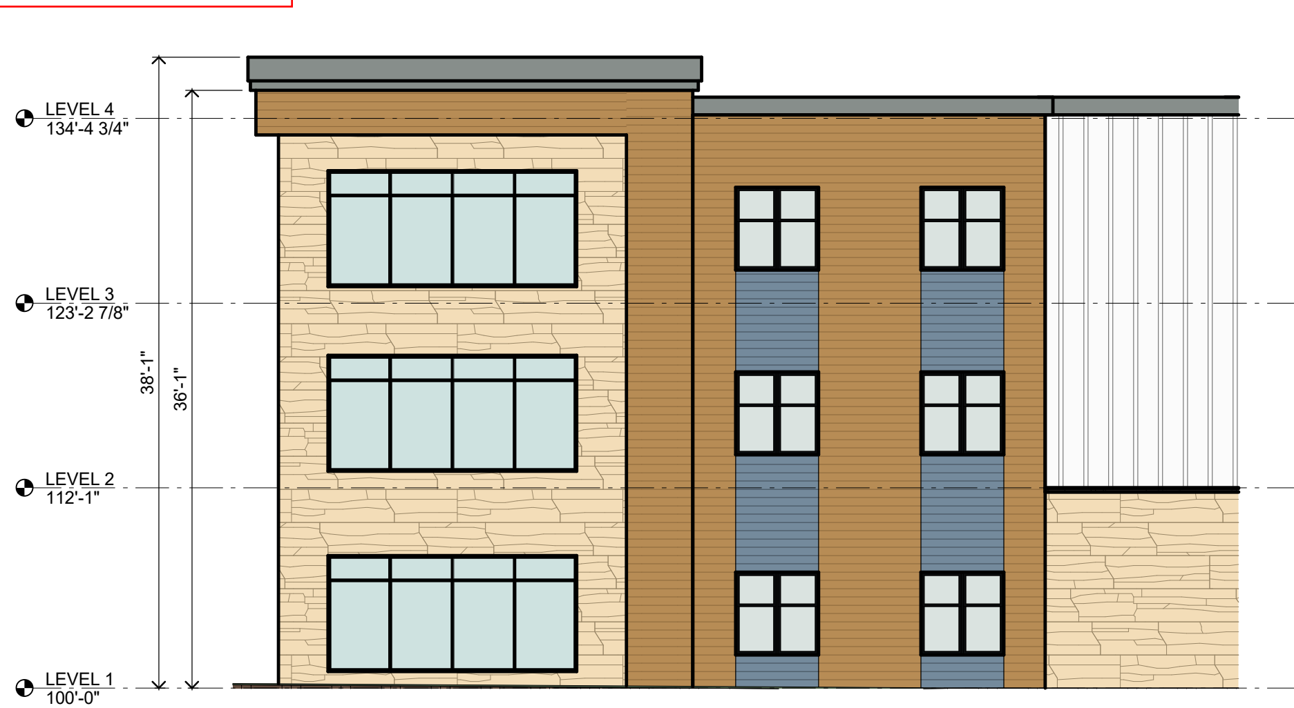
B2 CARE CENTER - ELEVATION 2 1/8" = 1'-0"
