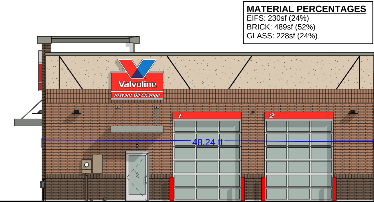
1 EXTERIOR ELEVATION (REAR) North Scale: 1/8" = 1'-0"
